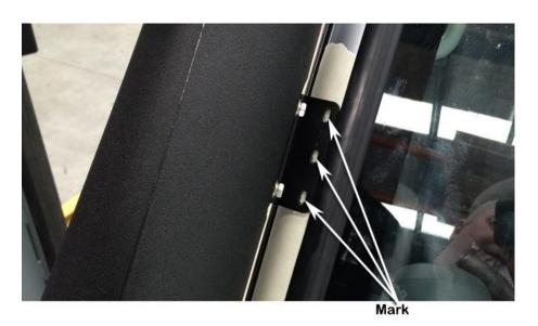
Mark the centre of each of the marked slots positions on the A-pillar, Drill a pilot hole at each of the three marked hole centres.
