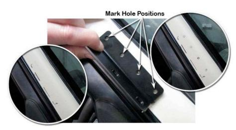
Drill a pilot hole in the centre of each marked hole position and use a step drill to drill to 8mm diameter.
