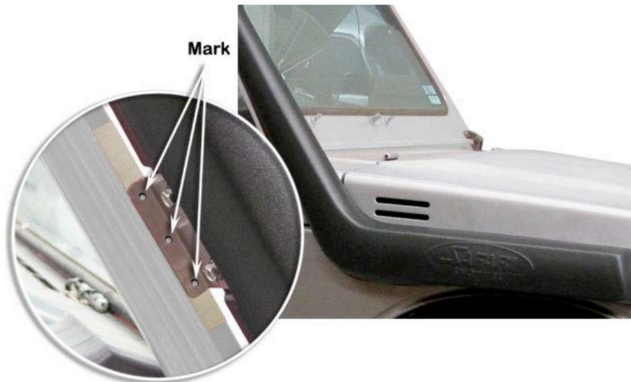
**8** Remove the snorkel body (Item 1) from the vehicle and remove the upper mounting bracket (Item 3) from the snorkel body.
