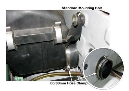
Loosely install the 60/80mm hose clamp (item 11) to the air entry hose and install the air cleaner base, fasten into position with the standard mounting bolts.
